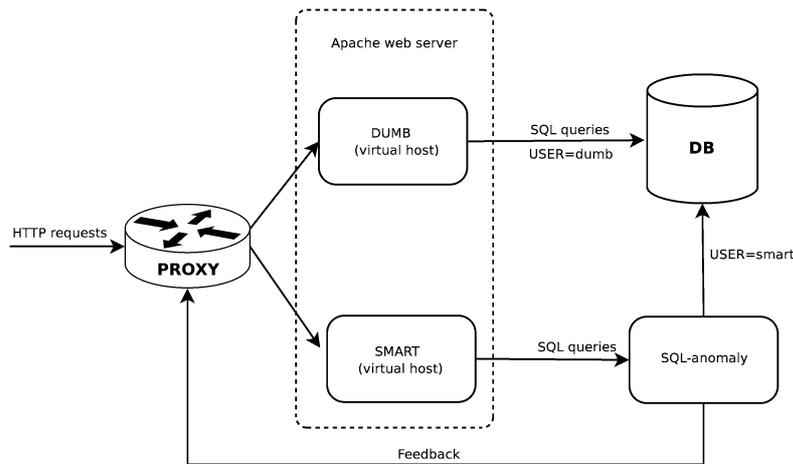
Fig. 6. Testbed architecture.
